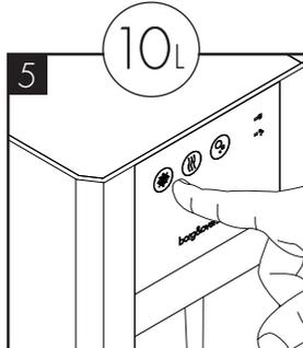
Flush through approximately 10 litres of water. Check and adjust the CO2 pressure accordingly.
