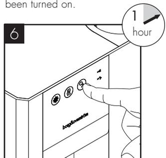
It will be necessary to leave the machine for up to 1 hour for sparkling water to develop, by absorbing the CO2.
